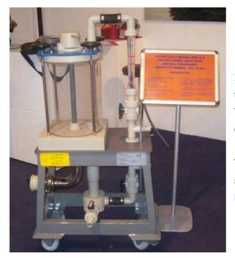
It works only if it is connected in series with the filter pump through special valves. The recovering takes place through the resin, contained in the filter unit.
